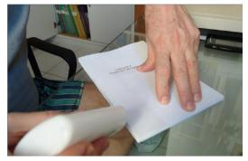
QUANDO A COLA SECAR, RETIRA-SE O CADERNO DA PRENSA. PASSA-SE COLA SOBRE A BORDA INTERNA DO CADERNO PARA A COLAGEM DA CAPA.
